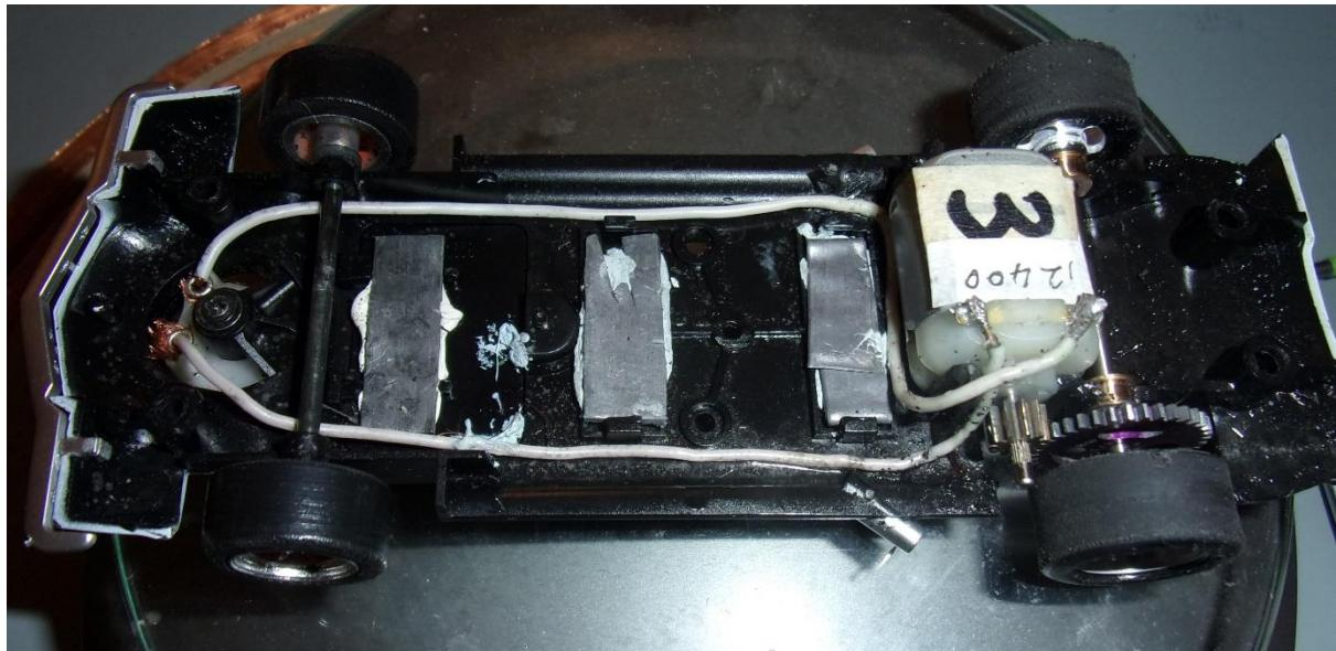
▲The optimum set-up; Rear track should ideally be 60 mm and the overall weight circa 86 gms with the chassis as above weighing 55 gms±
