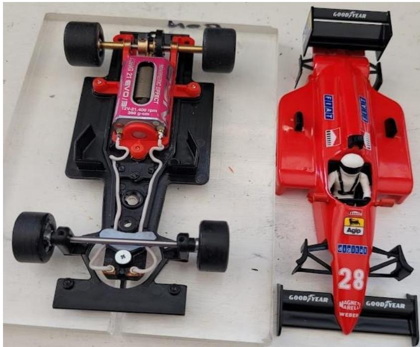
NB. Mike L uses all four motor-pod fixing screws which seems to help...
