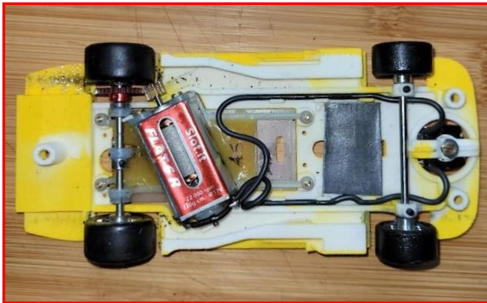
**NB.** Slot.it Metric Screws M2.5x6mm required for Carrera – Part No: SIHC89 whilst Ron recommended substituting the (front) Motor pod fixing screws with Slot.it Metric Screws 2.2x5.3mm Tapered Large Head – Part No: SICH54B – this was his recommendation for all cars using Slot.it Motor pods.
