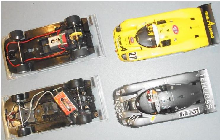
All Slot.it Group C cars need to be converted from 'Inline' to 'Anglewinder' configuration as illustrated and will be broadly similar irrespective of model -
