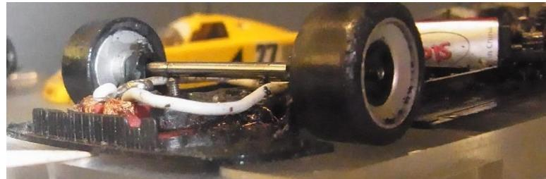
Note suspension at the rear of the motor-pod and the front axle adjustment which allows the wheels to rotate freely with just enough upwards travel to stabilise the car in the corners.
