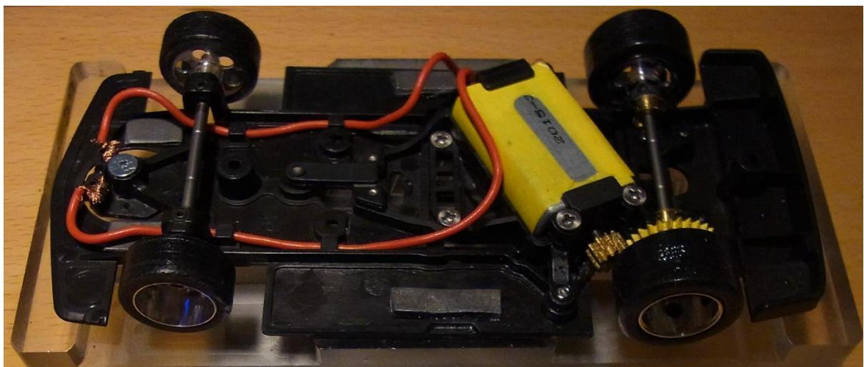
▲ This BMW 320 was set up by me – the front weights would probably be better centrally under the front axle whilst using a Slot.it motor mount would allow the side ones to be placed on the mount ahead of the motor.
