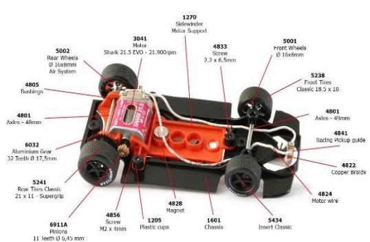
▲ More recent models have the NSR Shark 21.5K motor and come with screws to set / adjust front axle height.
