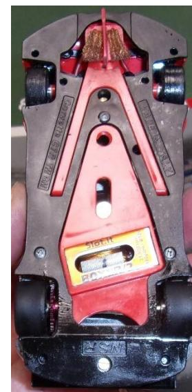
Note weight placed within the motor pod with a small amount in front of the front axle above the guide. A Slotting Plus Axle tube is used here – presumably to prevent flex although this is not common.
